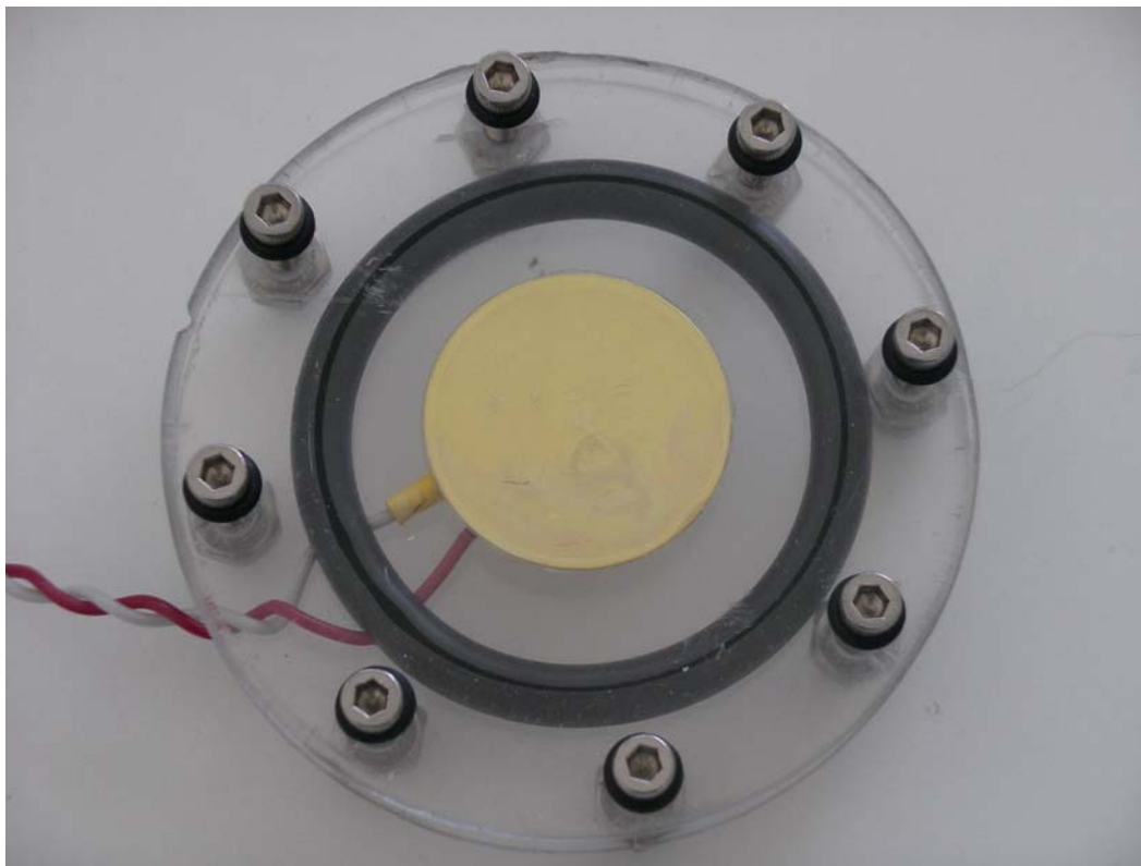
FIGURE 1. Completely assembled low-cost hydrophone. Note the wires going through the main O-ring and the smaller O-rings for each bolt.
